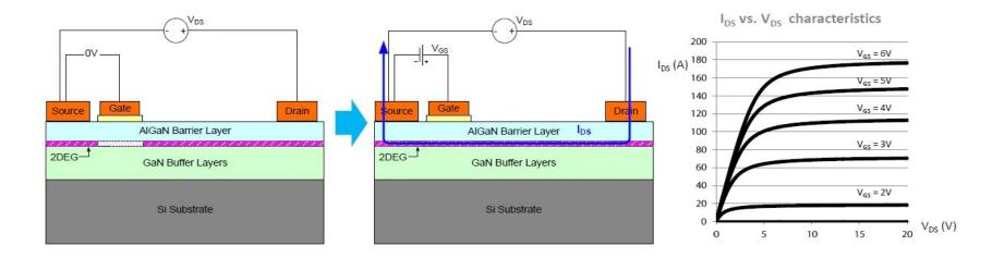
A GaN MOSFET power switch is built on a silicon substrate (Si or SiC), with a lateral two-dimensional electron gas (2DEG) channel formed on a AlGaN/GaN hetero-epitaxy structure that provides very high charge density and mobility; the enhancement-mode GaN device does not conduct when the gate drive is at zero but does conduct when the gate drive exceeds the threshold.
