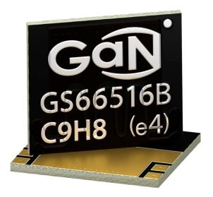
A representative GaN device is the "GaN Systems GS66516B", a 650V, enhancement-mode, GaN-on-silicon power transistor that combines high current, high voltage breakdown, and high switching frequency. On resistance is only 25mohm, and maximum drain-source current is 10A, while switching frequency can be as high as 10MHz and even higher.
