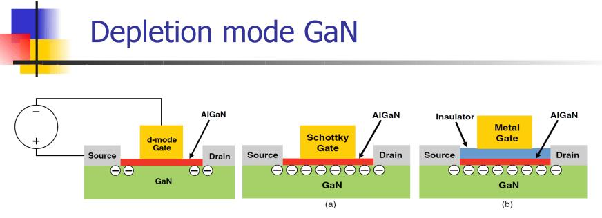
Cross section of a basic depletion-mode GaN HEMT with (a) Schottky gate, or (b) Insulating gate. In power conversion applications, d-mode devices are inconvenient because, at the startup of a power converter, a negative bias must first be applied to the power devices (such as GaAs and InP microwave devices). If this negative bias is not applied first, a short circuit will result between drain and source.
