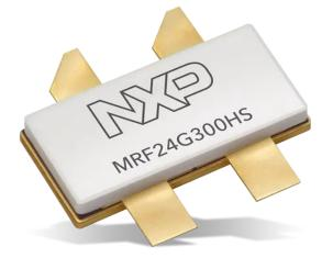
The new MRF24G300HS is a 50V GaN-HEMT with more or less similar characteristics but it has an efficiency of 73% at the same frequency and it can tolerate 20:1 of VSWR at all phase angles. Internally there are two sections so this device can be used in a single-ended or push-pull configuration.
