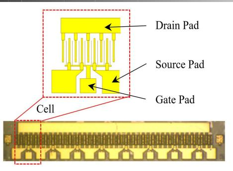
**GaN's primary advantage** over competing technologies is its **high power density**, which can be as much as 5X that of a comparable Si or GaAs device. In layman's terms, **that means five times the output power in an 80% smaller package size**.
